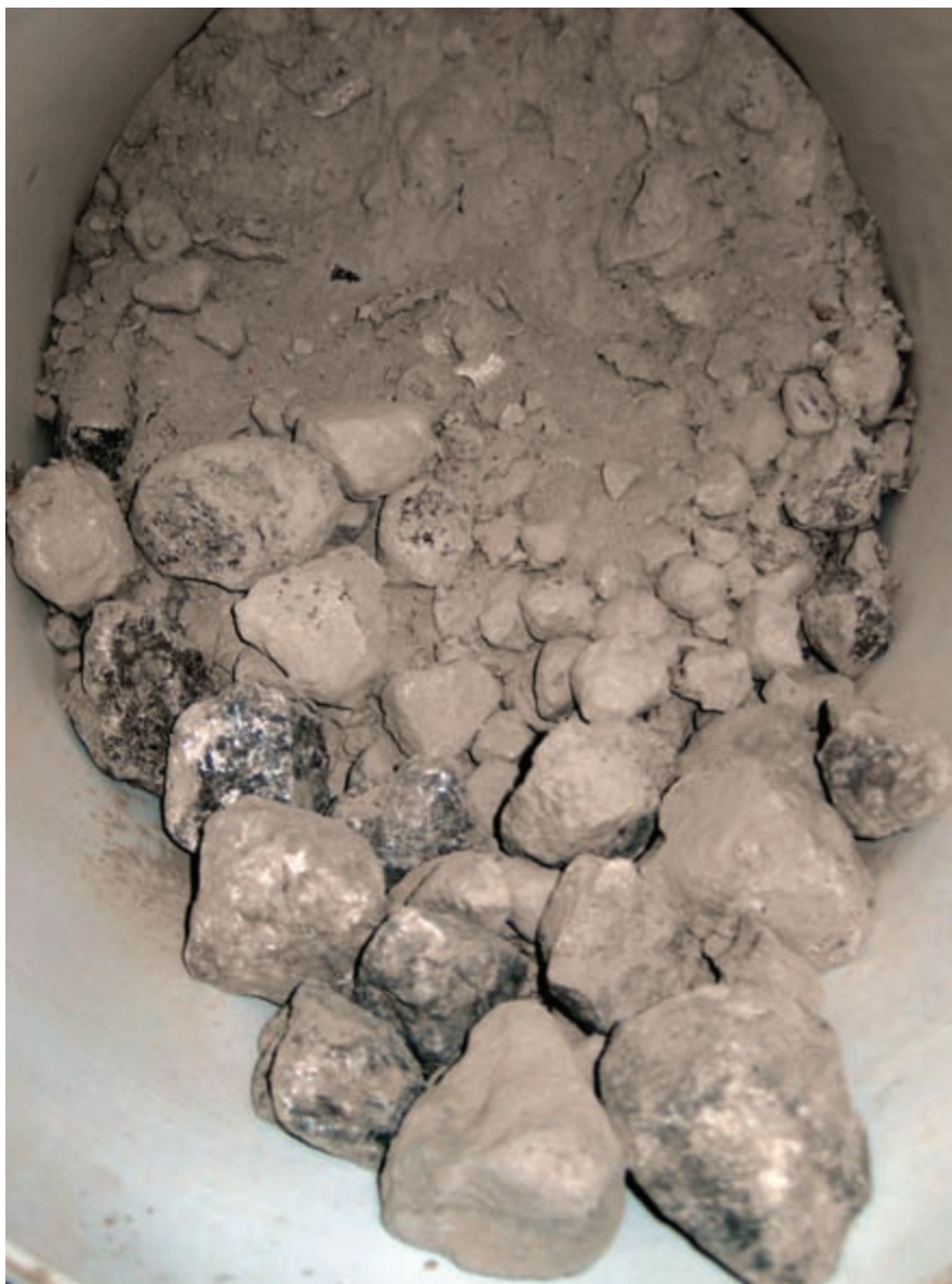
The approximately 2-inch-diameter gypsum rocks and fine powder were destroying the plant's heavy-duty rotary valves.
